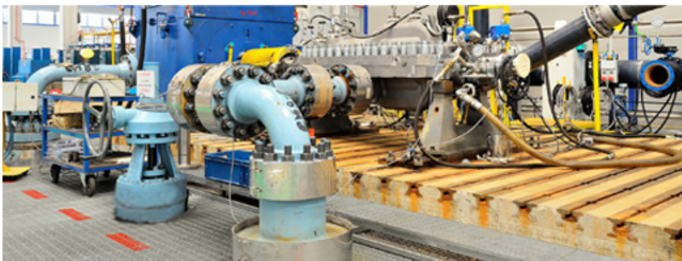
Multistage pump test assembly
